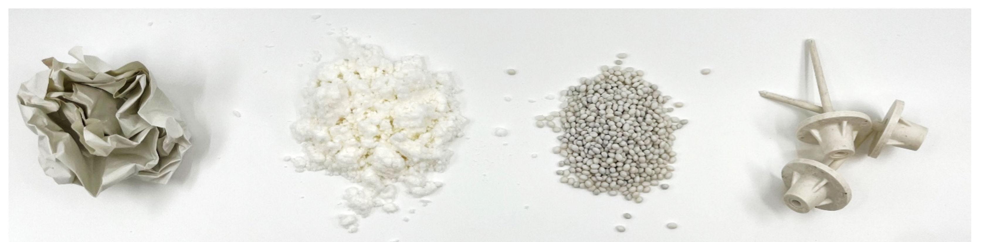
Figure 2: From paper via pulp and pellets to the final injection moulded part
